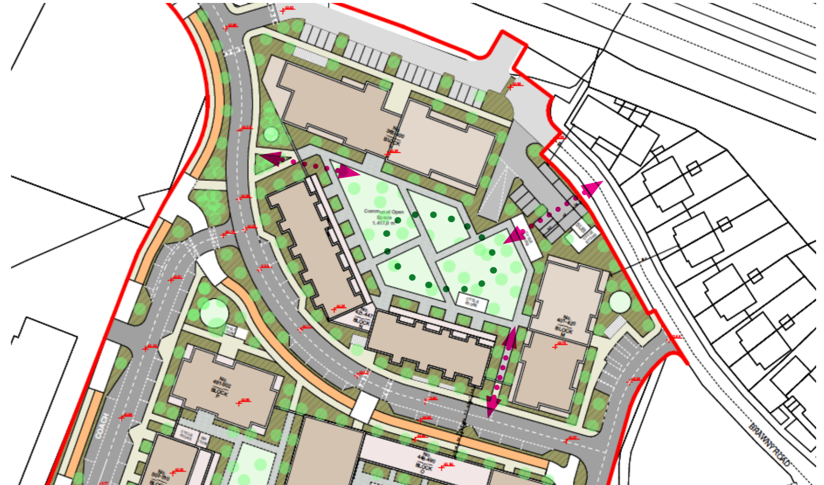
Part Site Plan showing blocks L, M and N, surface and bicycle parking, and the landscaped courtyard
