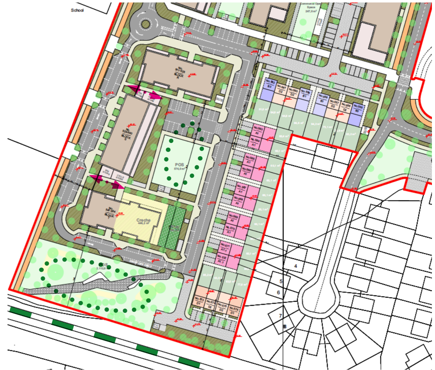
Part Site Plan showing apartment blocks R,S and T, two storey housing units, surface and bicycle parking, and landscaped open spaces
