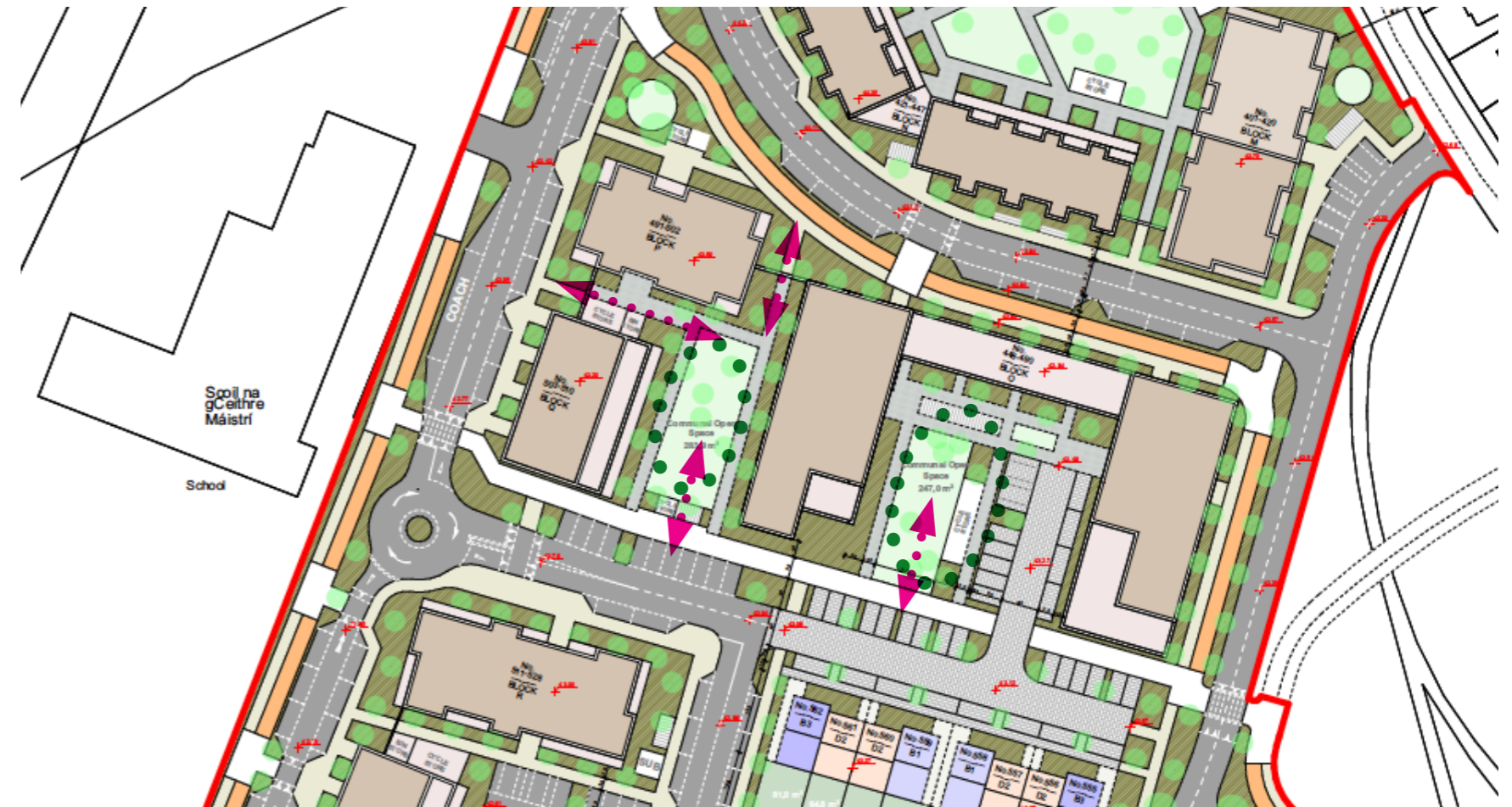
Part Site Plan showing blocks O,P and Q, surface and bicycle parking, and the landscaped courtyards
